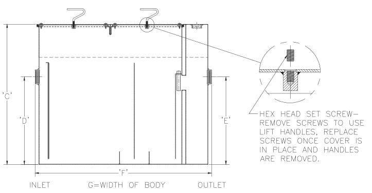
Location of inlet must be maintained at the 'D' dimension listed for each size.
