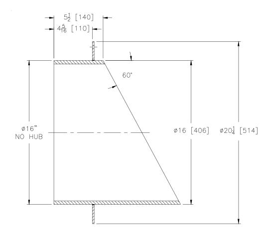
**ENGINEERING SPECIFICATION:** ZURN Z199-83 16 [406] Downspout Nozzle, Acid Resistant Coated fabricated steel body and wall flange.
