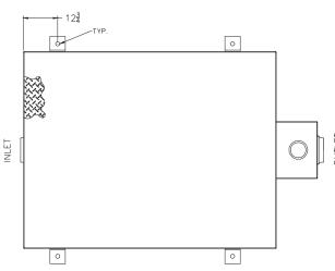
Note: Typ. 3 X 3 X 1/4 angle iron w/ 1/2" thru hole
