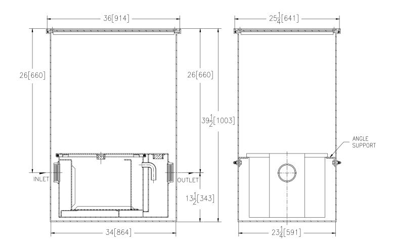
Size 600 **ENGINEERING SPECIFICATION**: ZURN Z-1170-95 Acid Resistant Coated fabricated steel recessing receiver, enclosed type, for recessed installation. Furnished with adjustable support brackets and gasketed non-skid cover recessed for 1/2 [13] thick tile with covered recessed lift handle. Complete with Z-1170 Greaseptor. For greaseptor specifications see Z-1170 drawing.
