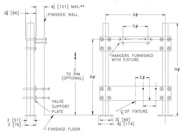
\*\* WITH STANDARD STUD LENGTH OF 6 [152]. #REFER TO ROUGH-IN GUIDE OF SPECIFIC FIXTURE FOR DIM.
