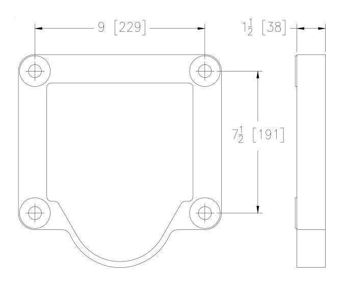
**ENGINEERING SPECIFICATION:** ZURN Z1200-FINFRAME-SJ ABS Finishing Frame for Siphon Jet System.
