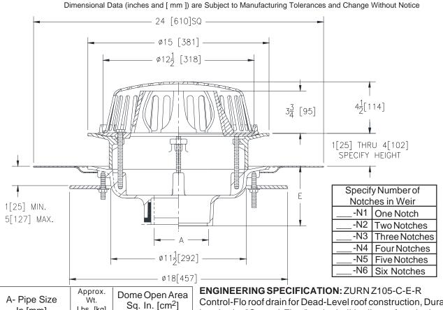
Control-Flo roof drain for Dead-Level roof construction. Dura-Coated cast iron body, "Control-Flow" weir shall be linear functioning with integral membrane flashing clamp/gravel guard, static extension, Poly-Dome, roof sump receiver and underdeck clamp. All data shall be verified proportional to flow rates. Each notch will allow 10 GPM of flow per inch of rain water build up above drain.
