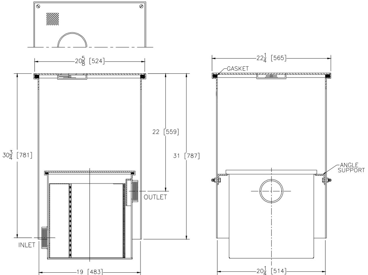
**ENGINEERING SPECIFICATION:** ZURN Z1181-92 Acid Resistant Epoxy Coated Recessing receiver equipped with adjustable support brackets and gasketed non-skid cover with recessed and covered lift handle. Complete with Z1181 solids interceptor for solids interceptor specifications see Z 1181 drawing.
