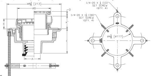
Note: Minimum K Dimension is Only Possible with -LR Option when using 6" [152] or 8" [203] Strainer
