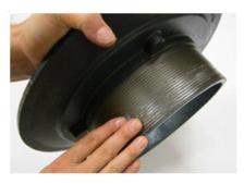
7. Apply white petroleum onto the external threads of the adjustable sleeve "J".
