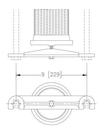
**ENGINEERING SPECIFICATION:** ZURN Z1210-29 Cast Iron test cap and straddle bar with gasket and adjustment bolt for water closet carriers.
