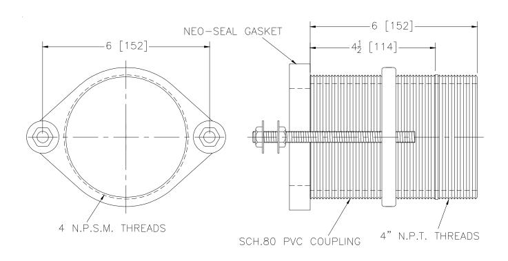
**ENGINEERING SPECIFICATION:** ZURN Z1210-F-79 Cast Iron adapter flange with fixture bolts and trim for floor mounted, back outlet closets, complete with adjustable PVC coupling and Neo-Seal gasket.
