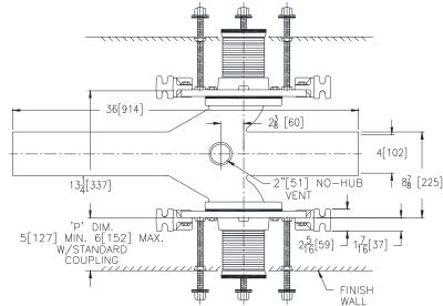
Feet bolted to floor using min. 1/2 [13] dia. bolts and back slots on carrier feet.
