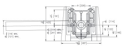
ZE1201-HL4-XH 4 [102] Hub & Spigot, Elongated Left Hand Inlet with Flow to Right ZE1201-HR4-XH 4 [102] Hub & Spigot, Elongated Right Hand Inlet with Flow to Left
