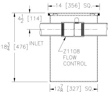
ENGINEERING SPECIFICATION: ZURN Z1108-81 Acid Resistant Coated interior and exterior fabricated steel access box with round openings for use with GT2700-35 grease interceptor recessing receiver, complete with gasketed non-skid secured cover.
