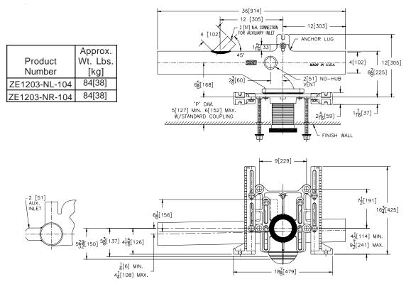
**ENGINEERING SPECIFICATION:** ZURN ZE1203-104() Adjustable, horizontal siphon jet water closet "Rigid System" with 4 [102] No-Hub connections. Complete with Dura-Coated cast iron right hand or left hand main fitting, with 2 [51] vent, adjustable gasketed face plate, universal floor mounted foot supports, corrosion resistant adjustable ABS coupling with integral test cap, 2 [51] auxiliary inlet, fixture bolts, trim, and stud protectors. Rear anchor tie down and bonded "Neo-Seal" gasket.
