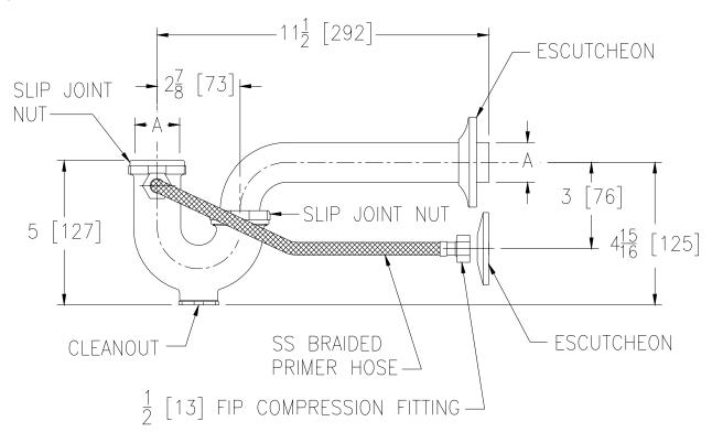
A - Pipe Size 1 1/2 [38] **ENGINEERING SPECIFICATION:** ZURN Z1021-WL Water Saver Trap Primer, chrome plated polished cast brass body with cleanout, one piece waste elbow, 1 1/2 [38] slip nuts and washers, and reducing washer for 1 1/4 [32] sink tail piece hookup, escutcheons and stainless steel braided primer hose with 1/2 [13] FIP compression fittings.
