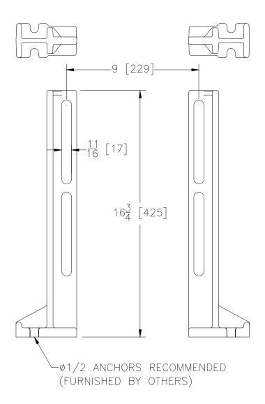
**ENGINEERING SPECIFICATION:** ZURN Z1210-M Dura-Coated cast iron floor mounted foot supports and support hardware. (For P-Dim. 10 [254] - 18 [457]. See Water Closet Carrier specification for reference)
