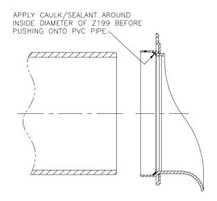
PUSH Z199 ONTO PVC PIPE, THEN INSERT AND TIGHTEN (3) SET SCREWS 120° APART FOR PIPE SIZES 2, 3, 4 & 5 INCH. (4) SET SCREWS, 90° APART FOR PIPE SIZES 6, 8, 10 & 12 INCH. —
