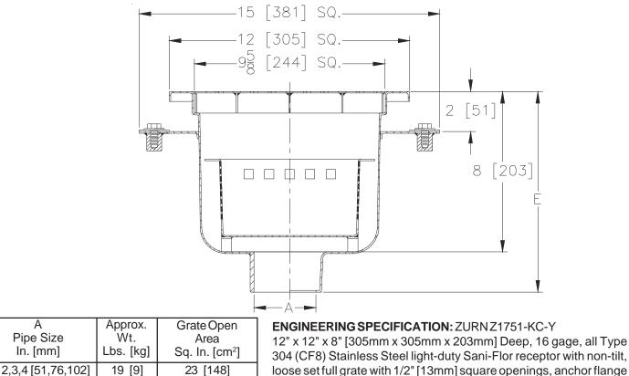
304 (CF8) Stainless Steel light-duty Sani-Flor receptor with non-tilt, loose set full grate with 1/2" [13mm] square openings, anchor flange with seepage holes and clamp collar, and sediment bucket.
