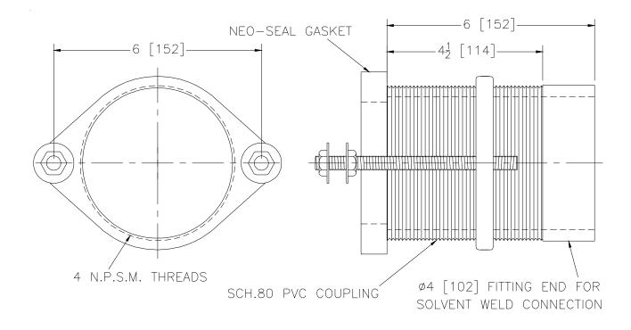
**ENGINEERING SPECIFICATION:** ZURN Z1210-F-78 Cast Iron adapter flange with fixture bolts and trim for floor mounted, back outlet closets, complete with adjustable PVC coupling and Neo-Seal gasket.
