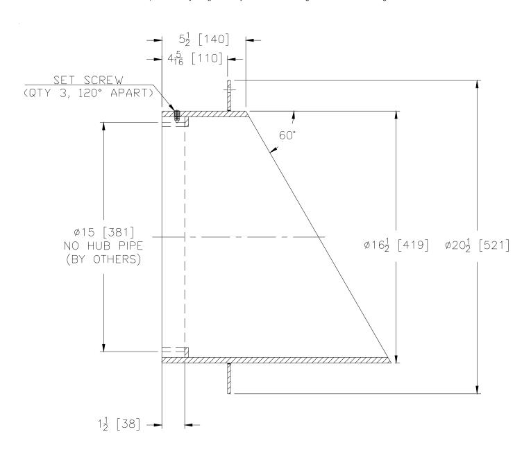
**ENGINEERING SPECIFICATION:** ZURN Z199-91 15 [381] Downspout Nozzle with PVC connection, Acid Resistant Coated fabricated steel body and wall flange.
