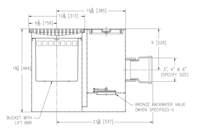
**ENGINEERING SPECIFICATION**: ZURN Z-1189-79 Dura-Coated fabricated steel body, interior and exterior with heavy duty Dura-Coated cast iron grate, visible double-wall outside trap seal, sediment bucket
