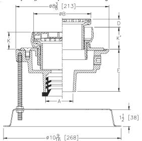
Note: Minimum K Dimension is Only Possible with -LR Option when using 6" [152] or 8" [203] Strainer
