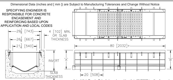
+Actual High Density Polyethylene channel length is 82 [2083] to allow for overlap, with frame attached the length is 84-1/2 [2146] with the exception of P.N. 2101P and 2130P.
