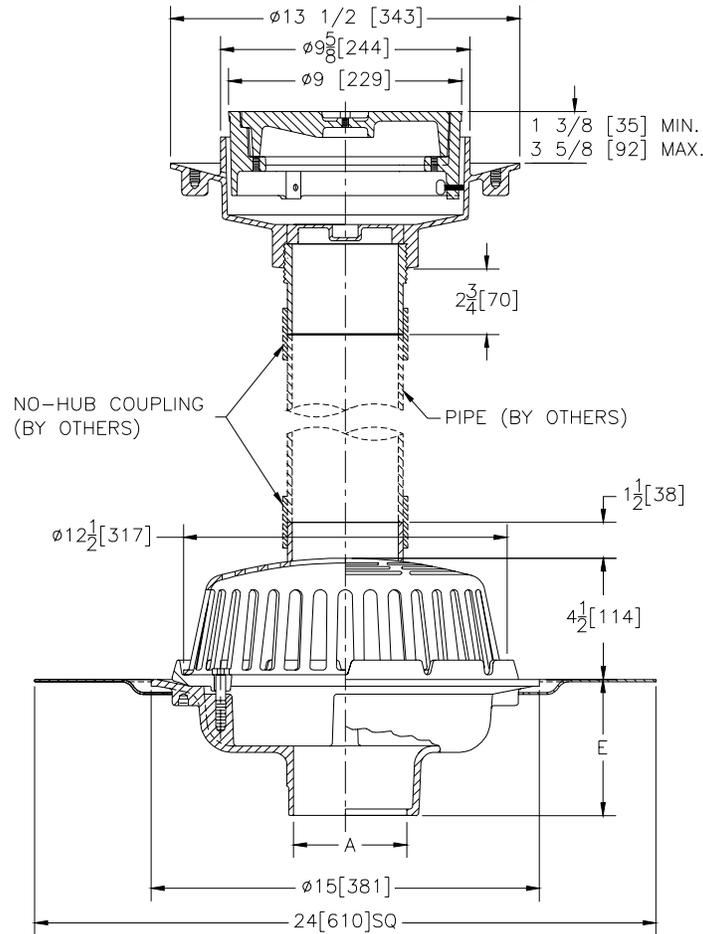
**ENGINEERING SPECIFICATION:** ZURN Z-100-145 15[381] Diameter roof drain. Dura-Coated cast iron body with combination membrane flashing clamp/ gravel guard, low silhouette dome, roof sump receiver in combination with upper floor cleanout, Dura coated cast iron body. gas and watertight ABS tapered thread plug, and round scoriated Dura-coated cast iron adjustable top, complete with membrane flashing flange.
