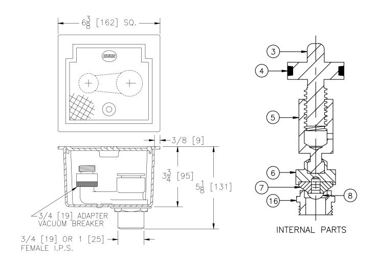
Approx. Wt. Lbs. [kg] **ENGINEERING SPECIFICATION:** ZURN Z1375-VB Encased, moderate climate ground hydrant, for flush with grade or finished floor installation. Complete with all bronze interior parts, replaceable bronze seat and seat washer, non-turning operating coupling with free-floating compression closure valve and 3/4 [19] adapter vacuum breaker, D.C.C.I. box and scoriated hinged cover.
