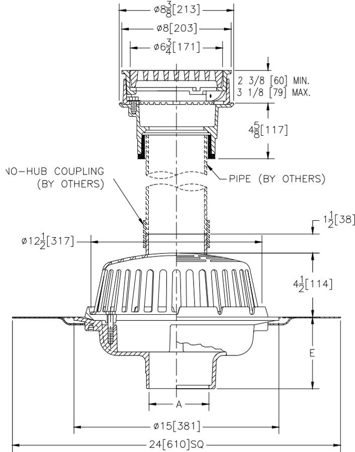
**ENGINEERING SPECIFICATION:** ZURN Z-100-144 15[381] Diameter roof drain. Dura-Coated cast iron body with combination membrane flashing clamp/ gravel guard, low silhouette dome, roof sump receiver in combination with upper floor drain, Dura coated cast iron body with bottom outlet, seepage pan and combination membrane flashing clamp, and frame for adjustable extension with heavy duty slotted cast iron grate.
