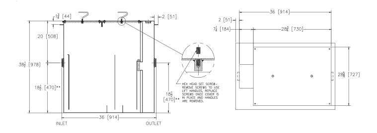
\* Location of inlet must be maintained at the '18-1/2 [470]' dimension listed for size.
