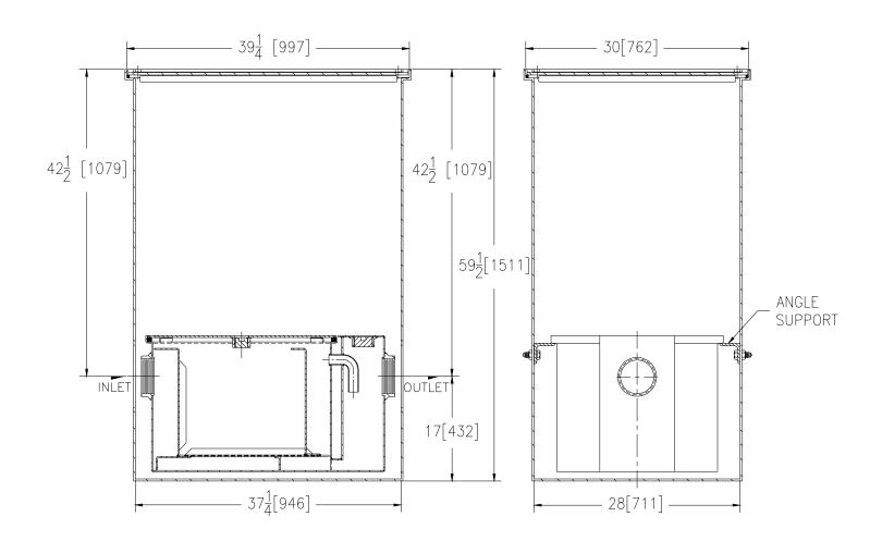
Size 800 **ENGINEERING SPECIFICATION**: ZURN Z-1170-90 Acid Resistant Coated fabricated steel recessing receiver, enclosed type, for recessed installation. Furnished with adjustable support brackets and gasketed non-skid cover recessed for 1/2 [13] thick tile with covered recessed lift handle. Complete with Z-1170 Greaseptor. For greaseptor specifications see Z-1170 drawing.
