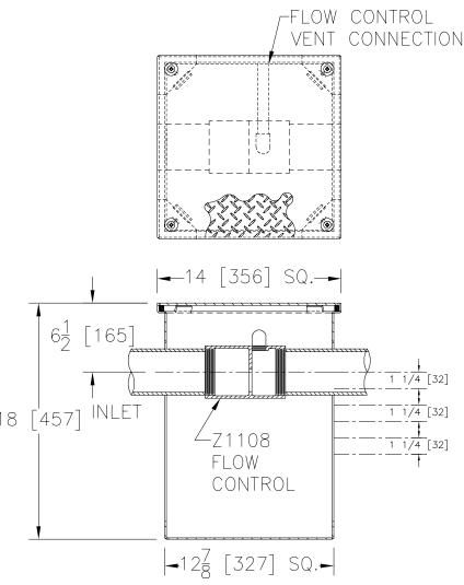
ENGINEERING SPECIFICATION: ZURN Z1108-80 Acid Resistant Coated interior and exterior fabricated steel access box with slotted openings for use with Z1170-600 grease interceptor recessing receiver, complete with gasketed non-skid secured cover.
