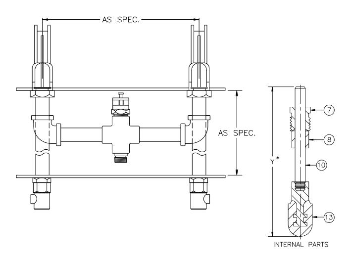
ENGINEERING SPECIFICATION: ZURN Z-1395-76 Exposed, non-freeze yard hydrants for hot and cold water, with Dura-Coated cast iron heads and lift handles with lock option. Bronze interior parts and galvanized steel casings with bronze valve housings and 1/4" IP drain ports in housing complete with single hose connection and atmospheric vacuum breaker.
