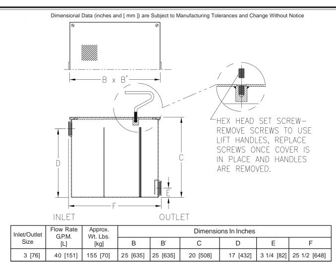
**ENGINEERING SPECIFICATION**: ZURN Z1185-113 Acid Resistant Coated interior and exterior fabricated steel lint interceptor, non-skid secured cover with removable lift handle, stainless steel lint intercepting secondary screen assembly and permanent primary straining baffle. Regularly furnished with high inlet and low outlet.
