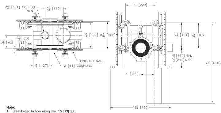
Feet bolted to floor using min. 1/2 [13] dia bolts and back slots on carrier feet.
