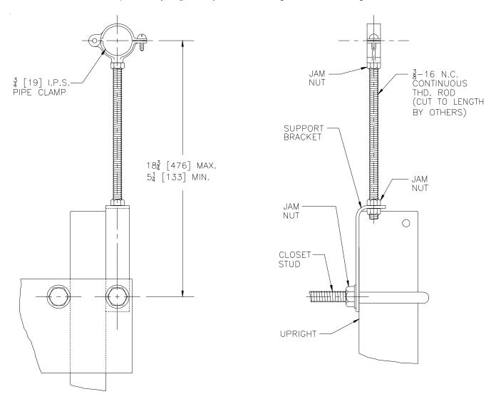
**ENGINEERING SPECIFICATION:** ZURN Z1210-58 Flush Valve Supply Support for Urinals.
