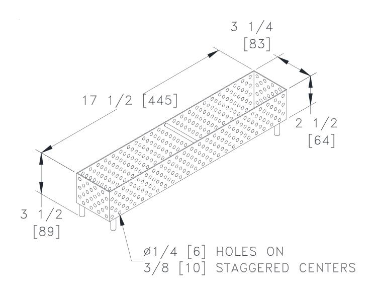
**ENGINEERING SPECIFICATION:** Zurn Z887-Y-75 6 x 20 [152 x 508] Shallow Sediment Bucket. Fabricated to fit inside of the Z887 6 x 20 [152 x 508] polyethylene catch basin. Perforated #18 GA. blue acid resisting epoxy coated carbon steel or stainless steel material on all sides allowing various objects and liquids to filter through. Complete with welded on handle for easy installation and maintenance.
