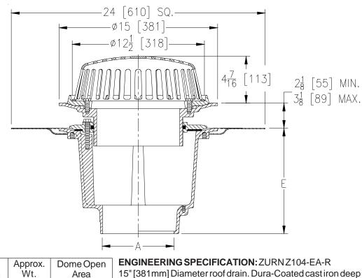
15" [381mm] Diameter roof drain. Dura-Coated cast iron deep sump body with combination membrane flashing clamp/gravel guard, adjustable extension, secondary clamping collar with o-ring, roof sump receiver and low silhouette Polv-Dome.
