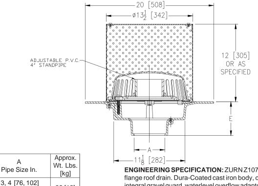
ENGINEERING SPECIFICATION: ZURN Z107-106 20 [508] Wide deck flange roof drain. Dura-Coated cast iron body, clamping collar with integral gravel guard, waterlevel overflow adaptor, adaptor plate, adjustable P.V.C. 4" standpipe, secured Poly-Dome strainer, and stainless steel gravel guard with solid secured cover.
