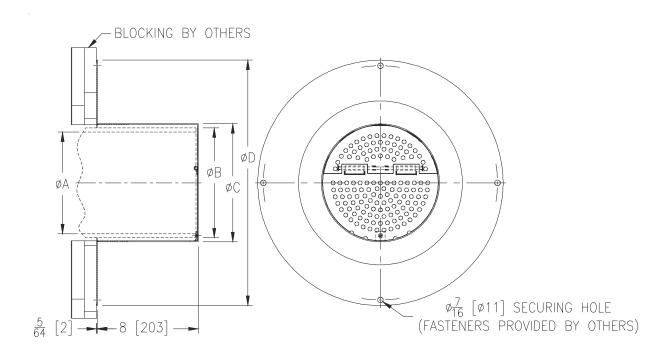
**ENGINEERING SPECIFICATION:** ZURN ZS199-DC-83 Downspout Cover with 8 [203] long, round fabricated stainless steel frame with fabricated secured perforated stainless steel hinged strainer, and wide flange.
